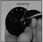
1. Remove external seals (Fig. 2B) with a screwdriver. Be careful not to tear or mar the
